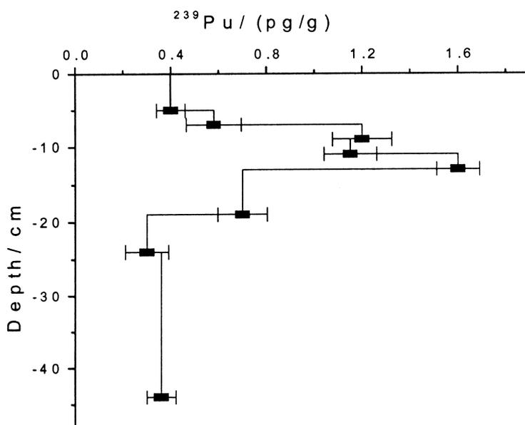
Figure 7. The concentration of  $^{239}\text{Pu}$  in the dry soil sampled in Gansu, China.
