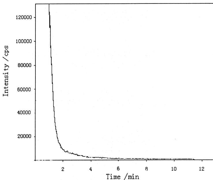
**Figure 5.** Elimination of memory effect of plutonium by rinsing with 0.025 mol/L oxalic acid in 0.15 mol/L nitric acid. Injection: 1 ng/mL  $^{242}\text{Pu}$  solution in 2% m/m nitric acid for 5 min, followed by 2% nitric acid for 2 min and then ( $t=0$  min), rinsing with acidic oxalic solution.
