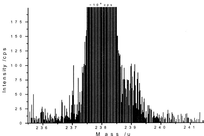
Figure 3. Inductively coupled plasma mass spectrum of uranium (236–241 Daltons).
