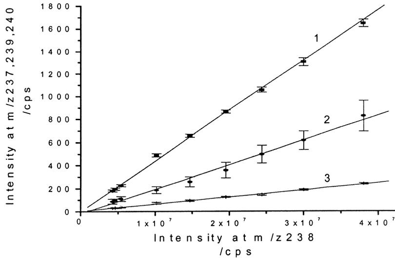
**Figure 4.** The dependence of signal intensity at  $m/z$  237, 239, and 240 with signal intensity at  $m/z$  238. Sample: uranium solution of different concentrations. Nebulizer: pneumatic nebulizer. 1,  $^{239}\text{I}/^{238}\text{I}$ ; 2,  $^{237}\text{I}/^{238}\text{I}$ ; 3,  $^{240}\text{I}/^{238}\text{I}$ .
