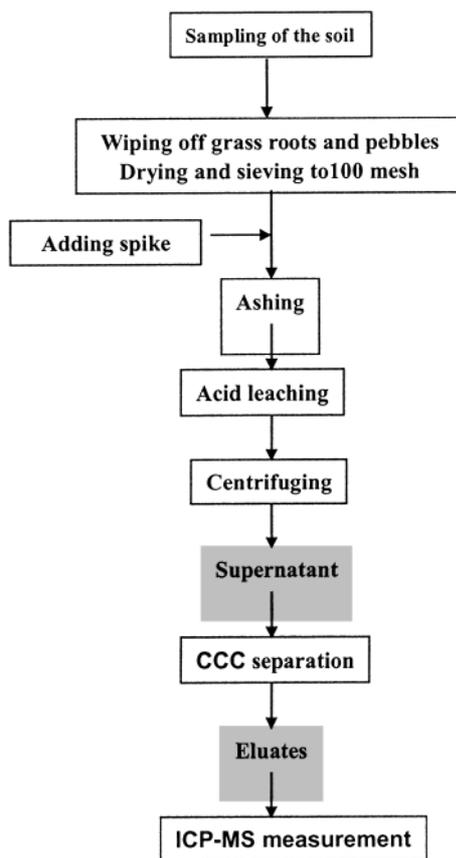
**Figure 1.** The analytical procedure for the soil.
